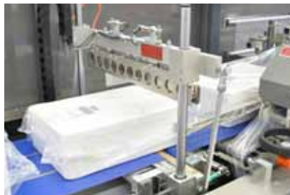
Universa 500 Servo: Perfect packaging results for highest requirements. With 7" widescreen Easy Touch-Panel.
