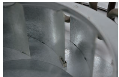
The ring-nozzle heating system ensures uniform heat transfer to the package contents.
