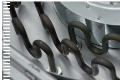
The ring-nozzle heating system ensures uniform heat transfer to the package contents.
